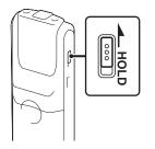
Slide the HOLD switch in the direction of the arrow in the recording or playback mode.
